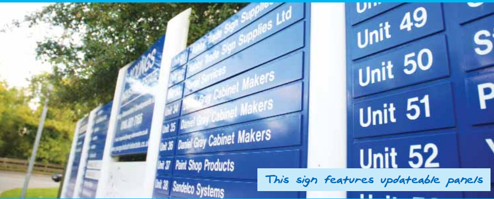
This inline sign features four trays, the middle section is made from two interlocking trays
